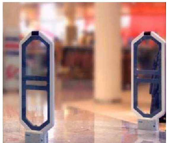
Magneto acoustic gate used for product surveillance
